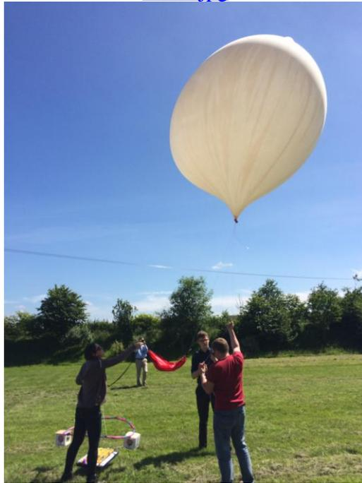
Figure 3 The helium balloon fully inflated and ready to launch
